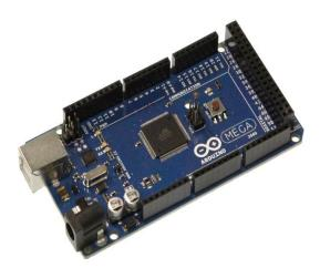
Figure 2: Photo of Arduino Mega 2560 microcontroller board
