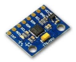
Figure 5: MPU 6050 sensor
